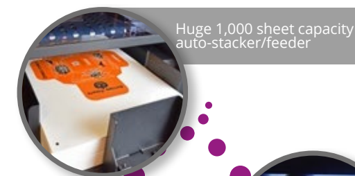
Front air blades and separating fingers assist media separation to perfectly feed every sheet
